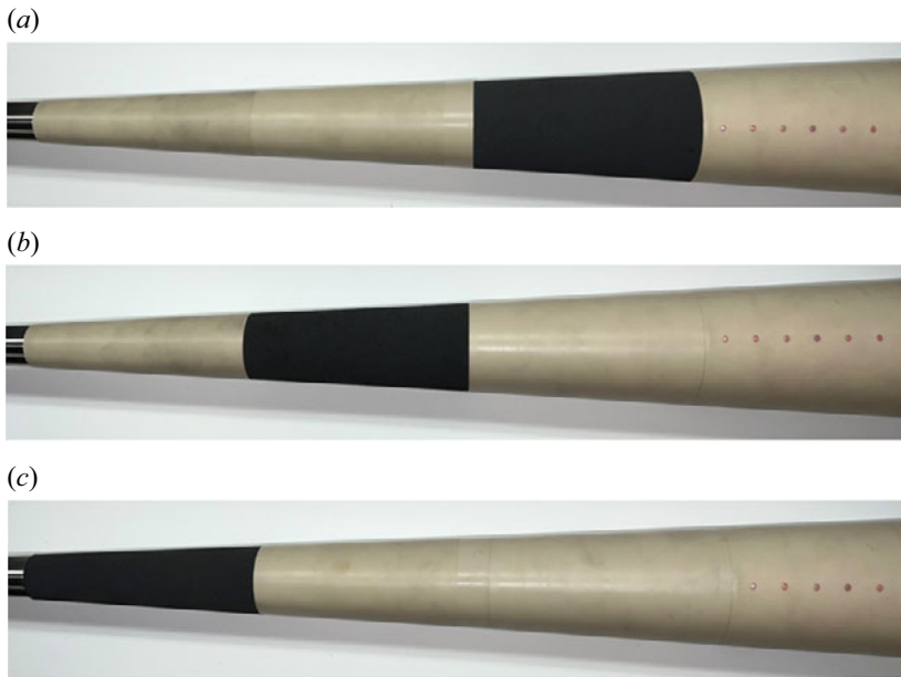
Figure 2. (a)–(c) Depict the 3^\circ half-angle cone with porous inserts installed at various locations.
