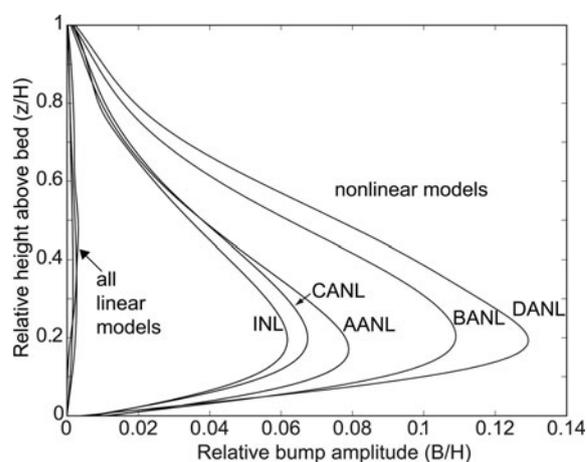
**Fig. 8.** Amplitude of the isochrone arch as a function of depth. Labels identify results from each model. The results for the corresponding models with a linear flow law are shown with the group label 'all linear models'. We express the arch amplitude ( $B$ ) as the distance above a curve that best fits each isochrone along the flank of the ice sheet. It is plotted as a function of the relative height of the isochrone ten ice thicknesses from the divide.
