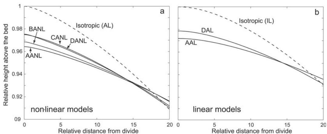
**Fig. 6.** (a) Steady-state surface profiles resulting from models using each of the four cone-angle profiles with a non-linear flow law, identified with the code given in Table 1. Dashed line shows the surface predicted by the model with isotropic fabric and a non-linear flow law. (b) Results for isotropic fabric and two cone-angle profiles using a linear flow law. All models are plotted relative to the ice thickness at the divide for the isotropic model.
