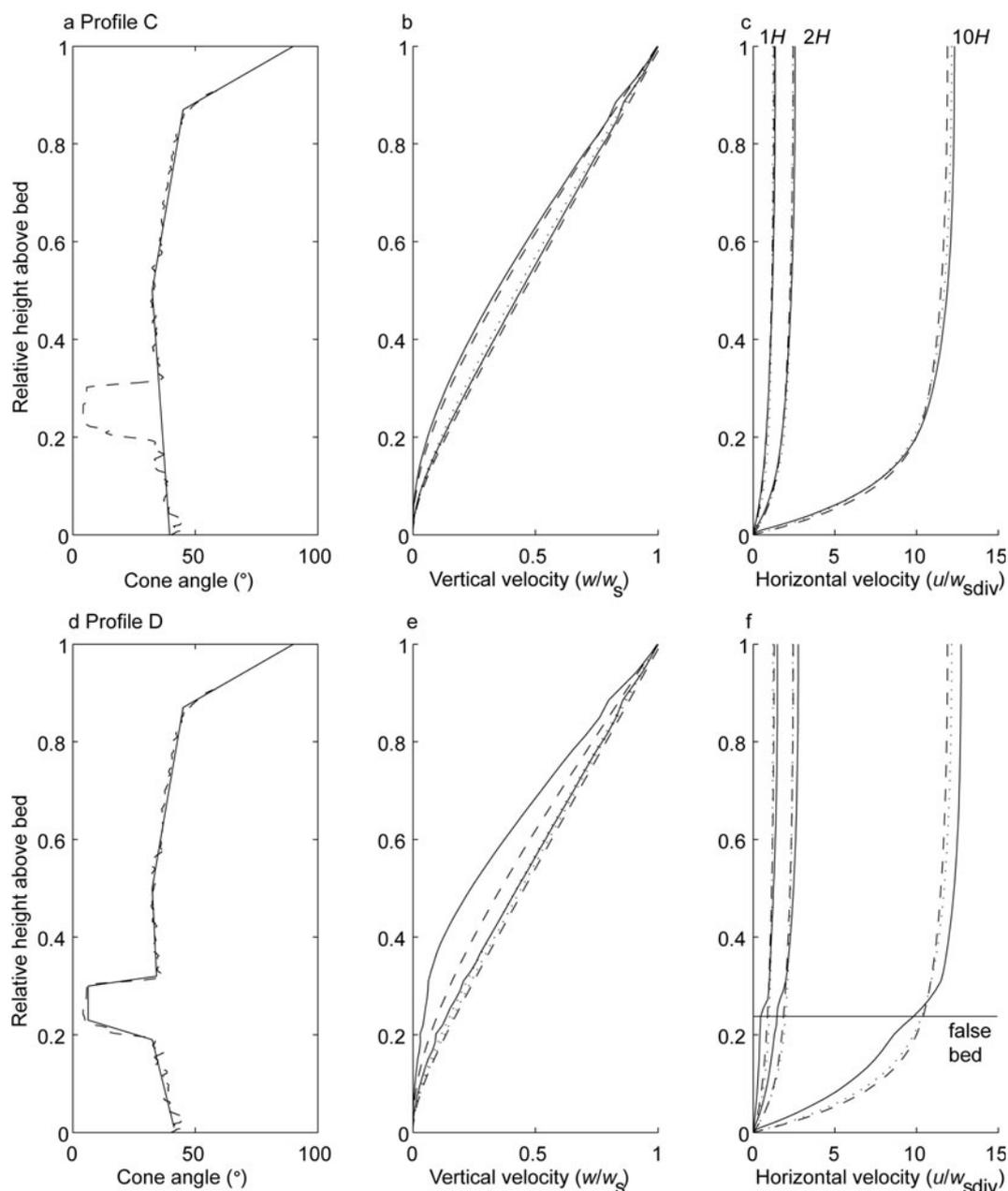
**Fig. 4.** Plot of the model results for two cone-angle profiles based on the sonic log for Siple Dome. The plotting conventions are the same as in Figure 3. The dashed line in (a) and (d) is the measured cone-angle profile for Siple Dome (personal communication, Greg Lamorey, 2003).
