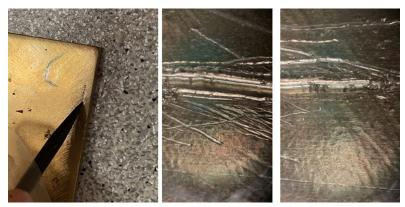
**Figure 12.** The author's simulation experiment of using an iron knife to engrave on a bronze plate (85 percent copper) and magnified images of the engraved lines. Photos by the author.
