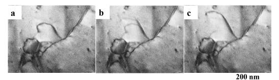
Figure 3. Bright field STEM image observation of dislocation slip in Cu thin foil at 600°C. (a:0s, b:0.5s, c:1.0s)
