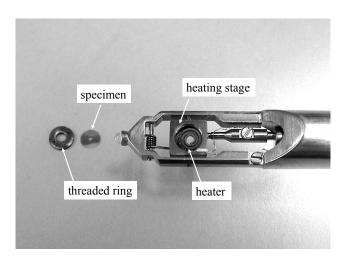
Figure 1. Double tilt specimen heating holder for standard TEM specimen(3mm dia.).
