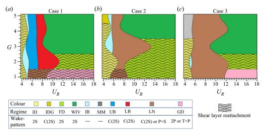
Figure 18. Identified FIV regimes, and associated wake patterns, for tandem cylinders corresponding to (a) Case 1, (b) Case 2 and (c) Case 3, on the  $U_R$ -G plane.
