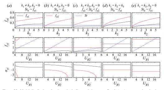
Figure 23. Modal distribution of various elastically coupled systems. Panels (a-c) correspond to the three configurations of Ding *et al.* (2020). Panel (*d*) corresponds to the configuration used by Kaja *et al.* (2013) and Cui *et al.* (2014). Panel (*e*) corresponds to the second configuration of Cui *et al.* (2014).
