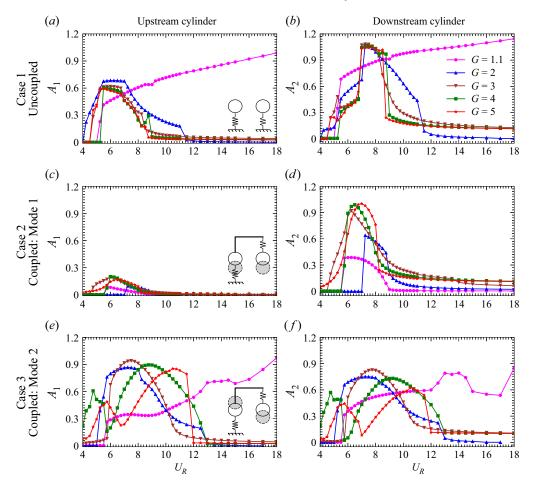
Figure 2. Variation of amplitude with reduced velocity  $(U_R)$  for (a,c,e) upstream cylinder,  $A_1$ , and (b,d,f) downstream cylinder,  $A_2$ : (a,b) Case 1, elastically uncoupled; (c,d) Case 2, elastically coupled, Mode 1; (e,f) Case 3, elastically coupled, Mode 2. Difference cases of gap ratio G are compared in each panel. The insets in (a,c,e) represent the configuration for Case 1, 2 and 3, respectively.
