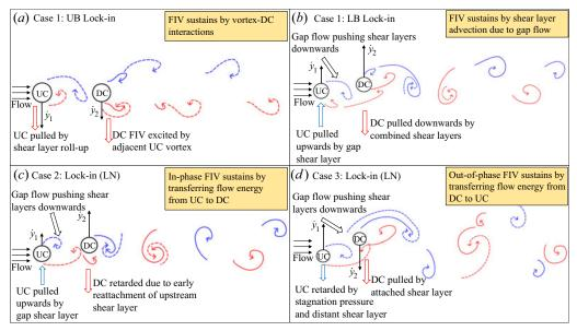
Figure 19. Schematic description of the lock-in mechanism for (*a*) Case 1, UB regime, (*b*) Case 1, LB regime, (*c*) Case 2, LN regime and (*d*) Case 3, LN regime.
