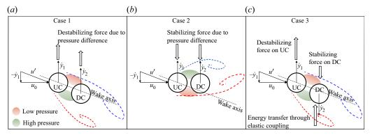
Figure 21. Schematic description of the mechanism of galloping for (a) Case 1, (b) Case 2 and (c) Case 3.
