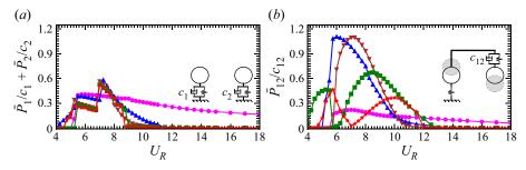
Figure 22. Energy harvesting potential for tandem cylinders using (a)  $P_1/c_1 + P_2/c_2$  as independent energy harvesters on uncoupled tandem cylinders in Case 1, and (b)  $\bar{P}_{12}/c_{12}$  as intermediate energy harvester between tandem cylinders in Case 3. Energy harvesting potential for all configurations is plotted in figure S6.
