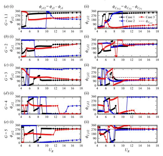
Figure 8. Here  $\phi_{y_{12}}$  (*a*i–*e*i) and  $\phi_{C_{T12}}$  (*a*ii–*e*ii) for G = 1.1 (*a*i,ii), G = 2 (*b*i,ii), G = 3 (*c*i,ii), G = 4 (*d*i,ii) and G = 5 (*e*i,ii). The dotted brown line in (ii) represent  $\phi_{C_{L12}}$ , corresponding to stationary tandem configuration.
