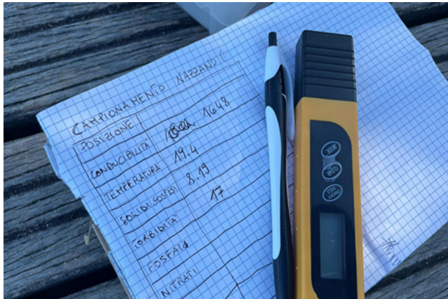
Figure 1: Instrument to monitor the temperature, conductivity and other parameters of water at a sampling point north of Rome (photograph by A Sud).
