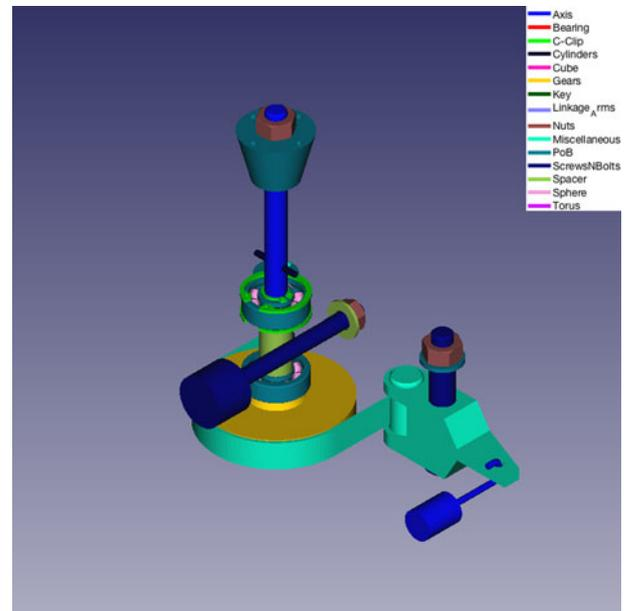
**Fig. 12.** The same model in Figure 11 with the removal of the carter.
