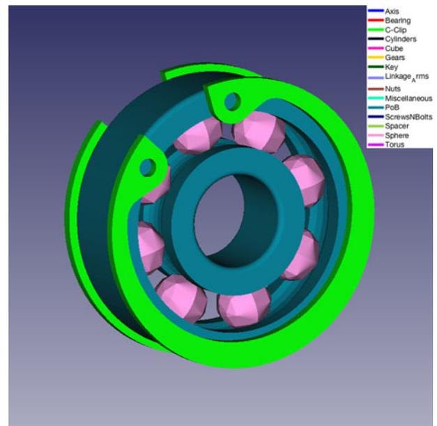
**Fig. 13.** A detail of the Mechanical Assembly Model in Figure 12. A bearing (made of two Part of Bearing and a series of Sphere-like parts) and C-Clips.
