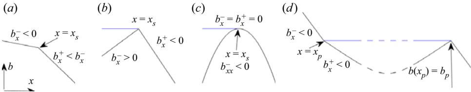
Figure 4. Different flavours of shocks and discontinuities in  $c$ : (a) ‘knickpoint’ shocks in flowing sections (§ 3.2), (b) seal shocks (§ 3.3), (c) smooth seals (§ 3.3) and (d) upstream ends of ponded sections, which can correspond to expansion fans but not to shocks (Appendix D).
