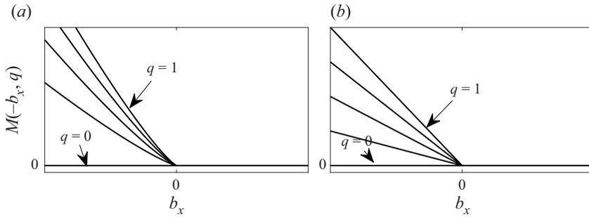
Figure 3. Melt rate  $M(-b_x, q)$  against  $b_x$  for  $q = 0, 0.25, 0.5, 0.75, 1$  for (a)  $\alpha = 0.5$ , (b)  $\alpha = 0$ ;  $M = 0$  when  $b_x > 0$ . Note that, although the two panels look similar,  $M$  in panel (a) is strictly convex for  $b_x < 0$  and continuously differentiable at  $b_x = 0$ , which has significant implications for shock formation in the model (2.11).
