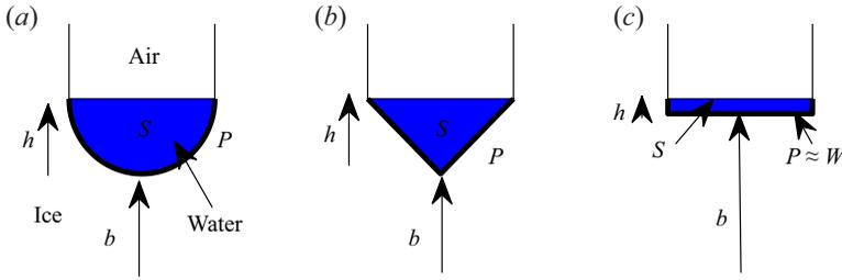
Figure 2. Cross-section shapes: (a) semi-circle ( $\alpha = \beta = 1/2$ ), (b) triangular ( $\alpha = \beta = 1/2$ ) and (c) fixed-width slot ( $\alpha = 0, \beta = 1$ ). Water with cross-sectional area  $S$  is shown in blue, wetted perimeter in heavy black. The qualitative nature of solution computed in § 4 depends on whether  $\alpha = 0$ .
