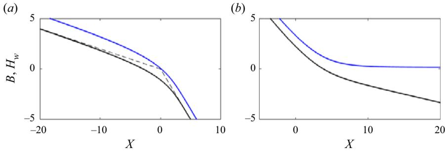
Figure 14. Boundary layer solutions with  $Fr = 0.575$ ,  $U = 1$ ,  $\alpha = 1/2$ ,  $\beta = 1/2$ ,  $q = 1$  for (a) the knickpoint boundary layer (Appendix B.1) with  $b_{0x}^+ = -1$  and  $b_{0x}^- = -0.2$  and (b) the pond entry boundary layer (Appendix D) with  $b_{0x}^- = -1$ ,  $b_{0x}^+ = \alpha b_{0x}^-/3$ . Black line shows  $B$ , blue shows  $B + \Sigma^\beta$ . The dashed lines in panel (a) show the outer solution as explained in § 2.4 of the supplementary material.
