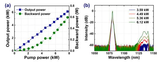
Figure 4. Basic output properties of the fiber amplifier employing the bidirectional pumping scheme: (a) power curve; (b) output spectra.
