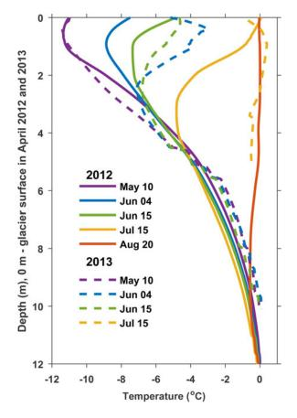
Fig. 3. Snow and firn temperature measured during 2012 and 2013.
