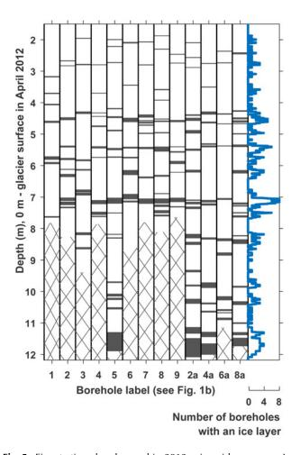
**Fig. 5.** Firn stratigraphy observed in 2012 using video surveys. Ice layers found in different boreholes are shown as horizontal black lines. The blue curve to the right illustrates the number of boreholes that indicated an ice layer at a specific depth.
