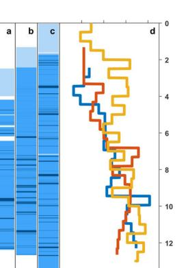
**Fig. 4.** Stratigraphy distribution observed in firn cores drilled in 2012 (a), 2013 (b) and 2014 (c). Different shades of the blue colour mark the depth intervals where snow (light), firn and ice (dark) were observed. Density distribution measured in cores in 2012–2014 (d).
