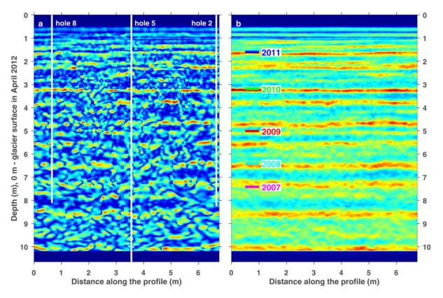
**Fig. 8.** Instantaneous amplitudes of the GPR data collected in April 2012. (a) radar profile crossing locations of boreholes 2, 5 and 8 (shown white, see Fig. 1b); (b) GPR data averaged in across-profile direction, also shown are the summer surfaces 2011–2007 (coloured labels) interpreted from a 500 MHz GPR profile Pelt2014.
