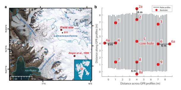
**Fig. 1.** (a) location of the study site at the Lomonosovfonna ice field with a map of Svalbard shown in the lower right corner. Also shown is the location of the Soviet expedition in 1965 Zinger1966; (b) the grid of boreholes and GPR profiles used in the study site. Note: the distances between boreholes 2 and 2a, 4 and 4a, 6 and 6a, 8 and 8a are not to the main scale.
