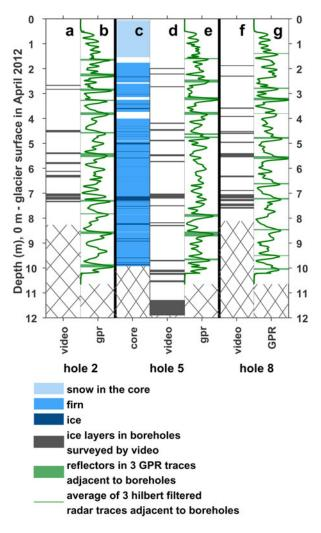
**Fig. 6.** Vertical profiles of firn stratigraphy derived in 2012 using different methods: firn core stratigraphy (c); ice layers recovered by video surveys in boreholes 2 (a), 5 (d) and 8 (f); reflectors and average instantaneous amplitude calculated for 3 radar traces sounded above boreholes 2 (b), 5 (e) and 8 (g).
