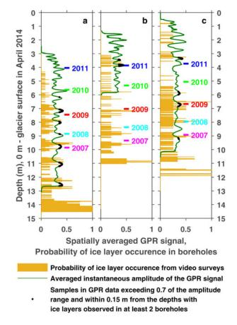
**Fig. 7.** Spatially averaged signals from the video and GPR data collected in 2012 (a), 2013 (b) and 2014 (c). Also shown are the summer surfaces 2011–2007 (coloured labels) interpreted from a 500 MHz GPR profile Pelt2014 and corrected for surface accumulation and gravitational firn compaction after April 2012.
