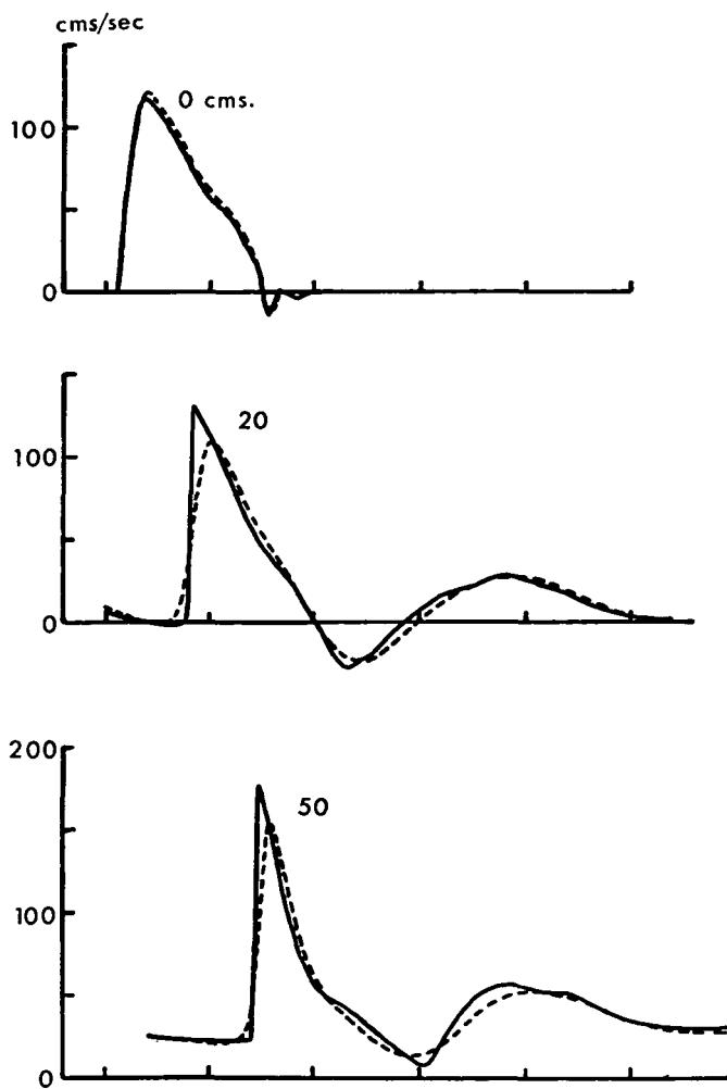
Fig. 3. Velocity-time profiles for the third cardiac cycle at the positions  $x = 0, 20, 50, 80, 100$  cm along the aorta as predicted by the one-dimensional blood flow model. The broken lines are the graphs obtained with coarse grid spacing, the solid lines are those obtained with fine grid spacing.
