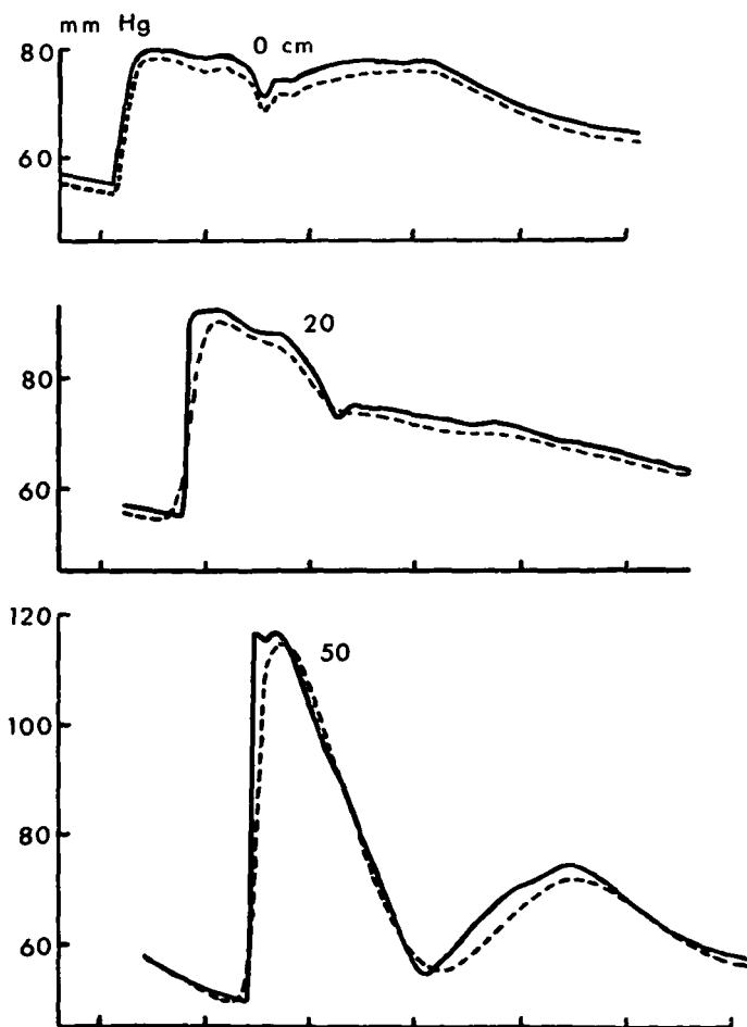
Fig. 2. Pressure-time profiles for the third cardiac cycle at the positions  $x = 0, 20, 50, 80, 100$  cm along the aorta as predicted by the one-dimensional blood flow model. The broken lines are the graphs obtained with coarse grid spacing, the solid lines are those obtained with fine grid spacing.
