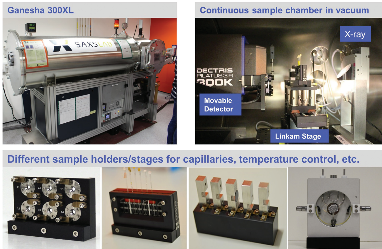
Figure 3: Top: Whole-vacuum SAXS/WAXS system at CNIE, including the Ganesha 300XL and moving detector. Bottom, left to right: Sample stages compatible with Ganesha. Sandwich cells, capillaries, and folded foil envelope can be used with the Linkam HFSX350-CAP (upper right) and enable temperature control across a wide range of samples.
