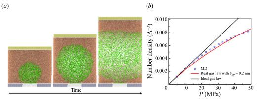
Figure 5. (a) The growth of unstable nanobubbles using  $J_{in} = 4.5 \times 10^{-15} \text{ kg s}^{-1}$ . (b) Equation of states measured from MD simulations (squares) in comparison with the ideal (black line) and real (red line) gas laws.
