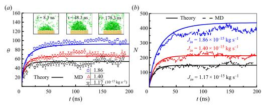
Figure 2. (a) Growth of contact angles to their equilibrium states for three different gas influxes  $J_{in}$  as given in the legend. The symbols represent MD results and solid lines are obtained by solving (3.5). The MD snapshots show the evolution of the simulated nanobubble for the case  $J_{in} = 1.86 \times 10^{-15} \text{ kg s}^{-1}$  at three different times. (b) Growth of the number of gas atoms in the bubble N(t) to the equilibrium state for the same three different gas influxes.
