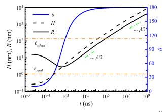
Figure 4. Unbounded growth of nanobubbles when the gas influx  $J_{in} = 5.2 \times 10^{-15} \text{ kg s}^{-1}$  is beyond the threshold influx  $J_{in,t} = 2.53 \times 10^{-15} \text{ kg s}^{-1}$ . For  $\ell_{real} \ll R \ll \ell_{ideal}$ , the scaling  $R \sim t^{1/2}$  is found while for  $R \gg \ell_{ideal}, R \sim t^{1/3}$ .
