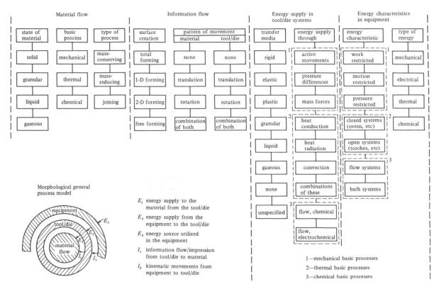
Figure 2. The morphological structure of material processes (Alting, 1978)
