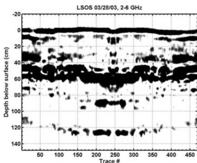
**Fig. 5.** FMCW radar scan, 2–6 GHz. Dark areas indicate strong reflections; light areas indicate no reflection. Distance scanned is approximately 3 m (trace 0–250). Measurement was made from left to right and then back again, illustrating the spatial variability present and the repeatability of the measurement.
