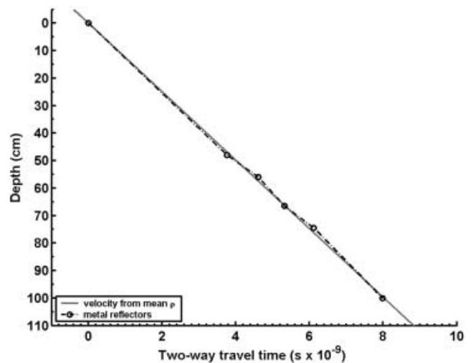
**Fig. 4.** TWT of large reflections caused by metal reflectors at various known depths.
