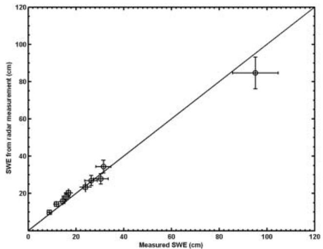
**Fig. 2.** Comparison of measured and modeled SWE. A vertical manual density profile was integrated to calculate the measured SWE, and the modeled SWE was found by using a typical dry snow density of  $\bar{\rho}_s = 250\text{ kg m}^{-3}$ . The vertical error bars indicate the error caused by choice of dielectric model when using radar measurements combined with a depth measurement, and the horizontal error bars indicate the estimated uncertainty in the measured SWE.
