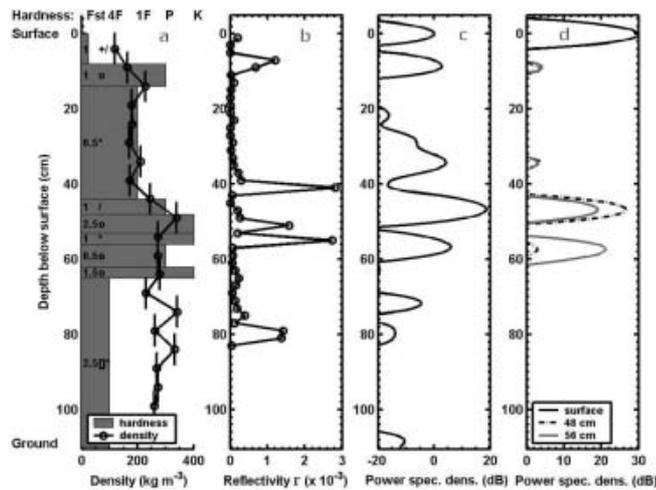
**Fig. 3.** (a) Manual snow pit showing visually identified layers, with hand hardness shown in gray (scale on top), and manual density measurements shown with circles (scale on bottom). Grain-size and type are indicated on the left. (b) In situ reflectivity calculated from snow-fork measurements. (c) Mean FMCW radar signal near snow pit. (d) FMCW radar measurements with metal reflectors at the surface, 48 and 56 cm.
