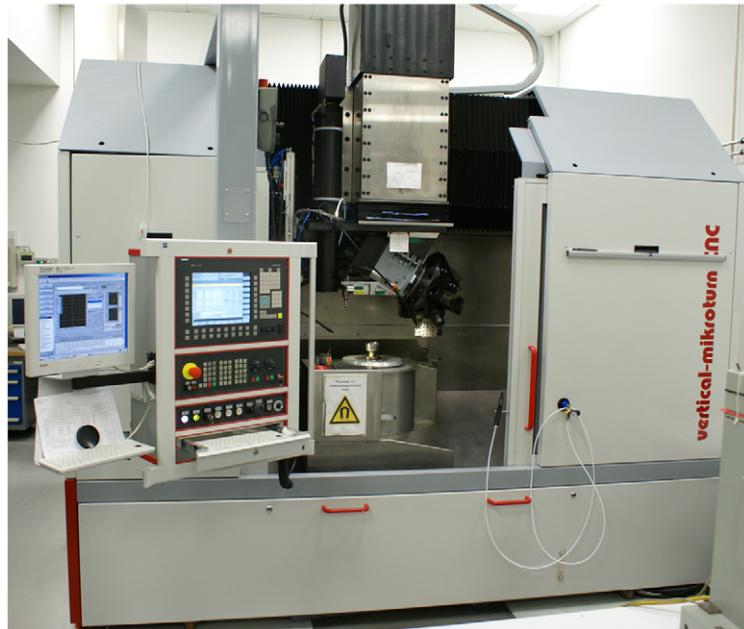
**Figure 12.** Self-adjusting alignment turning station for centring and aligning mounted lenses (Frank 2008); top – technical principle, translated into English by the authors; bottom – machine as built and used [Carl Zeiss Jena GmbH].
