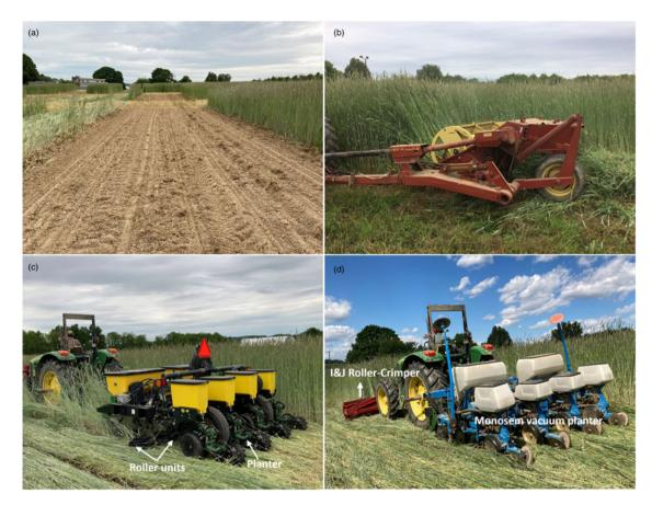
Figure 2. Cover crop termination method. (a) Cultivated field for soybean planting, (b) mowing cereal rye cover crop using haybine mower, (c) roller-crimping cereal rye cover crop using Dawn ZRX roller and Monosem planter, and (d) front-mounted I & J roller-crimper terminating cereal rye cover crop and rear-mounted Monosem vacuum planter in Kutztown, PA, USA.
