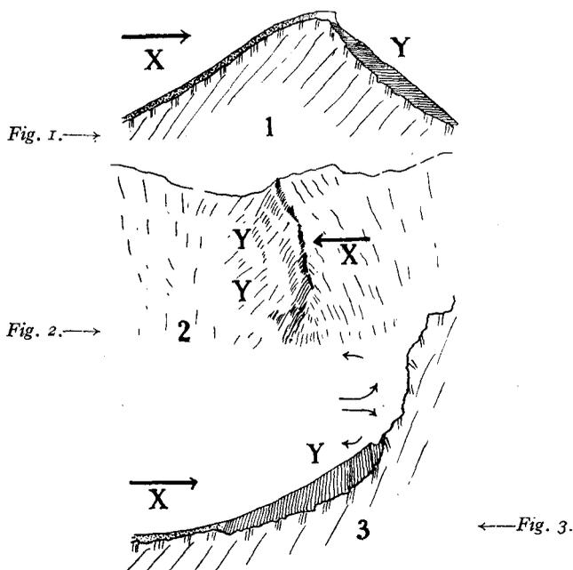
Fig. 3 shows quite a different effect. Here we have a not very steep slope culminating in a cliff; the wind is blowing straight against this cliff. Vortices are formed there and the wind loses its carrying power so that snow is thrown back to windward and deposited as a wind slab at Y. Fig. 5, Pl. III shows an example of this in the *Zillertal*, Tirol. The arrow denotes the scar of an enormous wind-slab avalanche which fell from there.
