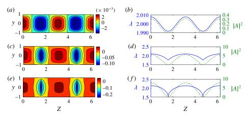
FIGURE 1. Morphology of vortex/TS wave ECS streak structure (a,c,e) and associated wall shear stress  $\lambda(Z)$  and TS wave amplitude  $|A(Z)|^2$  (b,d,f), where  $Z \equiv \epsilon z$ , with increasing magnitude of wave amplitude  $\mathscr{A}^2 \equiv \int_0^{2\pi/\beta} |A(Z)|^2 dZ$ :  $(a,b) \mathscr{A}^2 = 1$ ,  $(c,d) \mathscr{A}^2 = 20$ ,  $(e,f) \mathscr{A}^2 = 30$ . Adapted from Dempsey *et al.* (2016).
