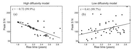
**Figure 4.** Theoretical plots of correlation between the peak sunspot number and the rise time (in years), obtained by introducing fluctuations in the meridional circulation. The two figures correspond to the high-diffusivity and the low-diffusivity models. Taken from Karak & Choudhuri (2011).
