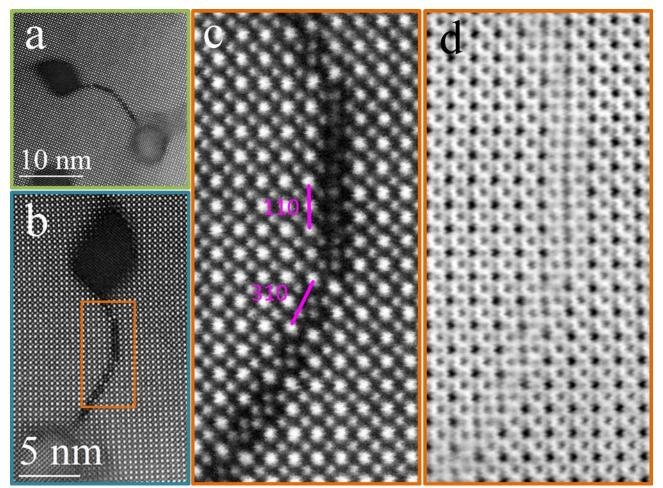
**Figure 1** (a) HAADF image of a plan-view 80 mol% LSMO-20 mol%  $ZrO_2$  sample showing two  $ZrO_2$  pillars connected by boundaries. (b) Magnified image of the boundary region shown in (a). Simultaneously acquired HAADF image (c) and ABF image (d) of the orange marked region in (b) including APBs with {110} and {310} boundary planes, respectively.
