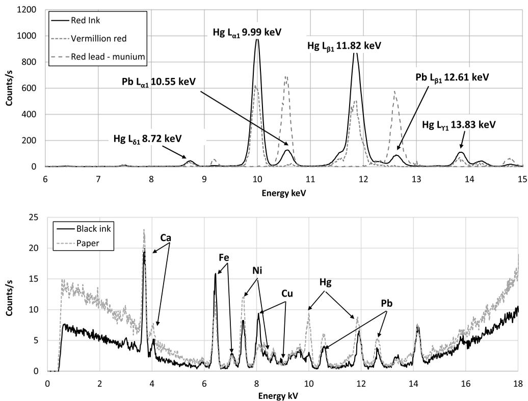
Figure 2 XRF spectra of the red ink (top) and black ink (bottom) used to print the manuscript. Comparison of the XRF spectrum of the red ink with the spectra of two pigments: vermilion (HgS) and minium (Pb<sub>3</sub>O<sub>4</sub>) shows that the red ink contains both pigments. The XRF spectrum of the black ink confirms its carbon-based nature. XRF spectra of black ink and background paper show the presence of the same trace elements in both spectra.
