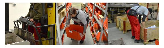
Figure 1. Field trial of passive exoskeleton Laevo V2.5 while stocking components and order picking.
