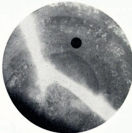
Fig. 9. Hole X, 1970. The bright areas consist of string that suspends a ball used to determine photograph scale; the ball is out of the field of view due to bore-hole curvature. The portion of the bed visible here has a diameter of about 105 mm.
