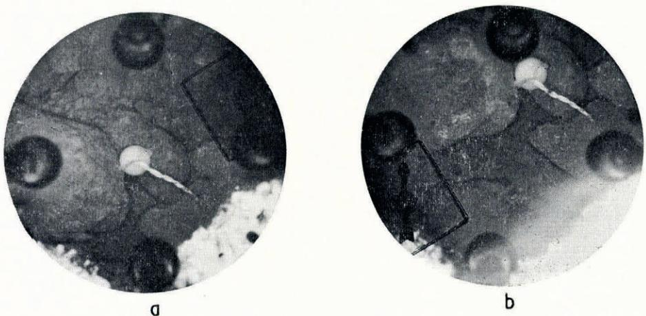
Fig. 3. Hole VI, 1969. (a) 7 September, 12.45 h. (b) 8 September, 10.50 h. The two bright areas in each photograph consist of ice attached to the bore-hole wall. Four lamp reflectors are seen, and a small nylon ball which rests on the bed. The portion of the bed seen has a diameter of about 87 mm.
