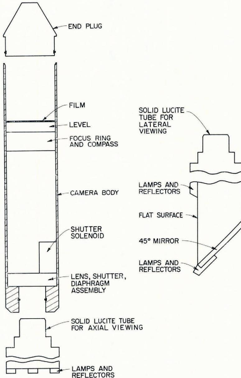
Fig. 1. Bore-hole camera including tube for axial viewing at left; tube for lateral viewing at right. The outside diameter of the camera is 51 mm.
