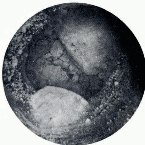
*Fig. 5. Hole X, 1970, showing the entire bottom of a bore hole. A cobbles and some finer material are seen embedded in the ice of the bore-hole wall. The portion of the bed seen has a diameter of about 105 mm.*
