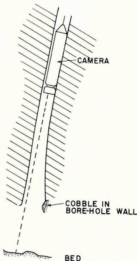
Fig. 10. Configuration of the bore hole and camera orientation as deduced from Figure 9. The bore hole was flared at the bottom during thermal drilling, and there is a gap between the base of the ice and the bed. The center of the camera is 0.9 m above the bed. The ice moves from left to right.
