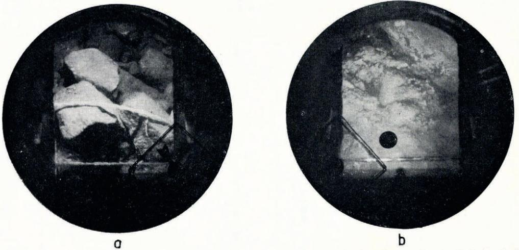
Fig. 6. (a) Hole VI, 1969, taken with the tip of the  $45^\circ$  mirror touching the bed. The string seen here is attached to the ball in Figure 3. Width of the foreground is about 38 mm. (b) Hole X, 1970, taken with the tip of the mirror 10 mm above the bed. Debris is seen in the basal ice. Width of strip photographed is about 41 mm.
