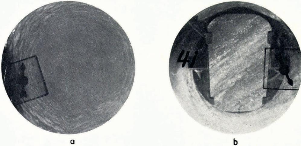
Fig. 8. (a) Hole VI, 1969. Bubbly ice. The notch in the hole wall at the bottom of the photograph was melted by the power cable during thermal drilling. Bore-hole diameter is about 59 mm. (b) Hole 16, 1967. Ice foliation. Width of strip photographed is about 30 mm.
