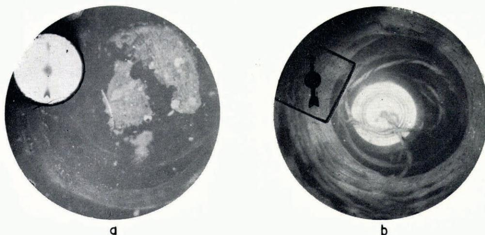
Fig. 11. (a) Hole T1, 1969. Thin layer of debris at the bottom of a bore hole. The maximum dimension of the larger patch of debris is about 45 mm. An early version of the compass was used. (b) Hole V3, 1969. Top of lost thermal drill. Bore-hole diameter is about 60 mm.
