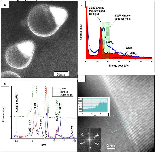
Fig. a. EFTEM image obtained using a 3.0 eV slit centered at 20 eV energy loss, showing solid/liquid "ice cream cone" nanoparticles.
