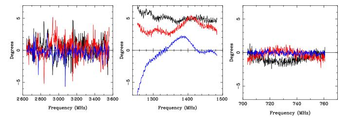
Figure 4. Modelled receiver polarisation parameters  $\epsilon_0$  (red),  $\epsilon_0$  (blue), and  $\theta_1$  (black). Left: the 10-cm system using PDFB4. Centre: the 20-cm multi-beam system using PDFB4. Right: the 40-cm system using PDFB3. The H-OH receiver is not displayed because it shows no evidence for feed cross-coupling.
