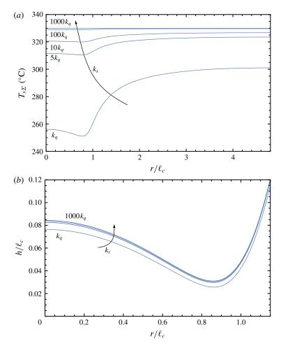
FIGURE 7. (Colour online) Effect of the variation of the substrate thermal conductivity  $k_s$  on the numerically predicted profiles of the substrate surface temperature (a) and the vapour film thickness (b) underneath a Leidenfrost ethanol drop of  $R = 1.37\ell_c$  with  $T_{imp} = 330\,^{\circ}\text{C}$  and the plate height ( $H_s = 4.5\,\text{mm} \approx 3\ell_c$ ) as in the experiment. The value of  $k_s$  for the quartz used in the experiment is denoted by  $k_g$ .
