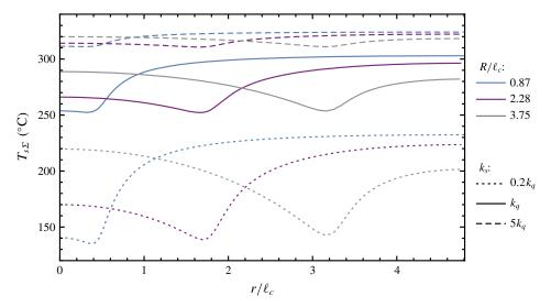
FIGURE 6. (Colour online) Numerically determined temperature profile at the top of the substrate underneath a Leidenfrost drop for different drop sizes and thermal conductivities of the substrate.  $H_s$  is taken at the value of the quartz plate height used in the experiment ( $H_s = H_q = 4.5$  mm).  $T_{imp} = 330$  °C and  $k_q = 1.4$  W m<sup>-1</sup> K<sup>-1</sup>, the thermal conductivity of quartz.
