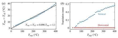
FIGURE 11. (Colour online) Temperature difference  $\Delta T = T_{imp} - T_{s\Sigma}$  across the quartz substrate in the absence of a drop (a) and the apparent translation relative to the reference interferogram (b).
