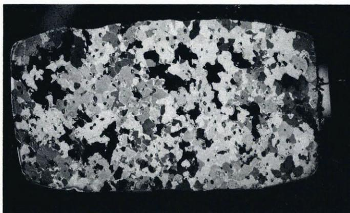
Fig. 9. Thin-section photograph of crystalline texture of ice specimen TC A2 between crossed polaroids after deformation in torsion-compression.  $\tau = 1.85$  bar and  $\sigma = 5.7$  bar; dimensions of the thin-section:  $8 \text{ cm} \times 4.5 \text{ cm}$ . The torsion axis was parallel to the direction containing the largest dimension of the thin section. The radial direction was perpendicular to the thin section.
