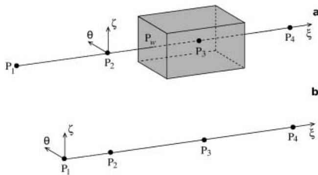
**Fig. 9.** (a) Four-point centred stencil for the approximation of diffusive fluxes on control volume faces and (b) four-point non-centred stencil for the approximation of diffusive fluxes at boundary points.
