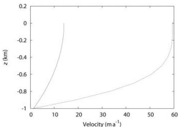
**Fig. 6.** Comparison between the vertical profiles of the longitudinal velocity of the simulation with constant viscosity (solid line) and variable viscosity (dashed line) in the centre of the domain with undulating bedrock. The sliding velocity is  $1.3 \text{ m a}^{-1}$  for the constant viscosity case and  $0.9 \text{ m a}^{-1}$  for the variable viscosity case.
