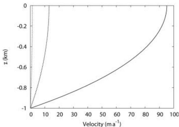
**Fig. 2.** Vertical profile of the longitudinal velocity for three kinematic viscosities:  $\nu = 10^{11} \text{ m}^2 \text{ s}^{-1}$  (solid line),  $\nu = 10^{12} \text{ m}^2 \text{ s}^{-1}$  (dashed line),  $\nu = 10^{13} \text{ m}^2 \text{ s}^{-1}$  (dotted line).
