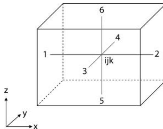
Fig. 1. Sketch of a three-dimensional control volume.
