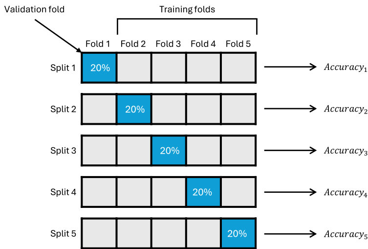
Figure 12. Illustration of k = 5 cross-validation. Each fold is used once for validation, while the remaining k - 1 folds are used for training. This reduces variance in validation error estimates and guides hyperparameter selection.
