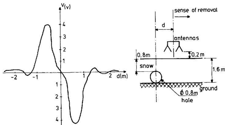
Fig. 5. Radiometer output signal when antennas move above a hole dug in a snow layer.
