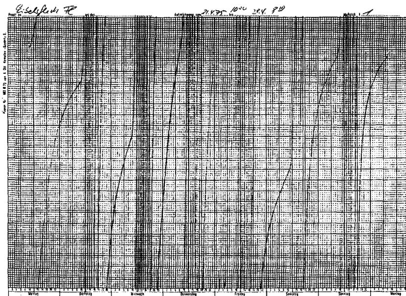
Fig. 4. A recording made by the lysimeter of the run-off from 25 m<sup>2</sup> of snow cover at 1 030 m a.s.l. in the Bavarian Alps, April 1975 (spring ablation). The 25 cm recording height corresponds to a collection of 75 l of liquid (c. 3 mm water column) when using a chart speed of 2 mm/h. (The recording which appears here has been photographically reduced.)
