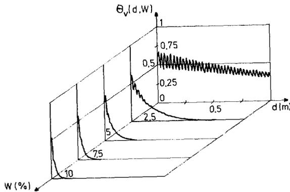
Fig. 4. Rate of power transmission  $\theta_v(d, w)$  through a homogeneous snow layer with thickness  $d$  and water content  $w$  in volume, placed on an infinite plane of muscular fibre at 4 GHz.
