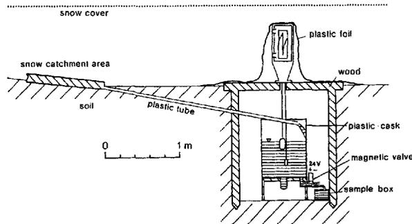
Fig. 1. The recording snow lysimeter.
