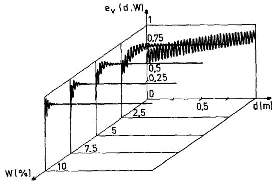
Fig. 2. Emissivity  $e_v(d, w)$  at the air-snow interface of a homogeneous snow layer with a thickness  $d$  and a water content  $w$  in volume, overlying an infinite plane of muscular fibre at 4 GHz.
