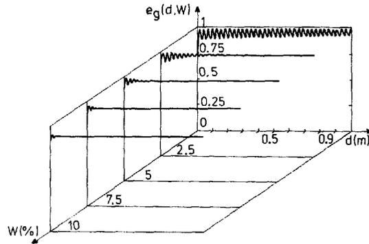
Fig. 3. Emissivity  $e_g(d, w)$  of snow with thickness  $d$  and water content  $w$  in volume at 4 GHz. Snow layer on sandy, wet ground.
