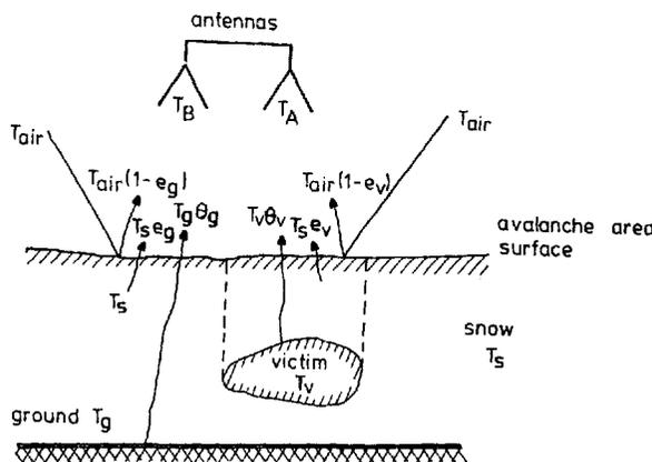
Fig. 1. Location of the antennas and of the human body in the snow.  $T_A$ ,  $T_B$  are the temperatures of the antennas,  $T_{air}$ ,  $T_s$ ,  $T_v$ , the real temperatures of the three materials involved.
