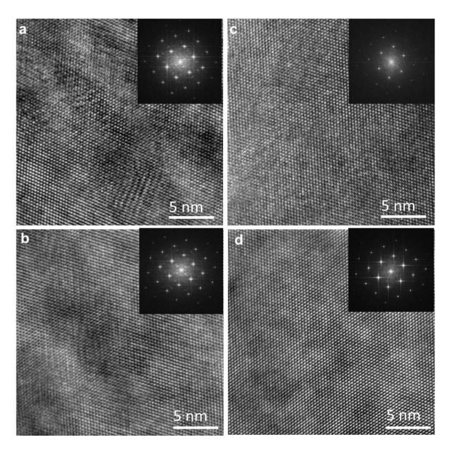
**Figure 1.** HRTEM images of Si specimens prepared by Ga FIB milling at 30 kV (top row) and 5 kV (bottom row). Insets are fast Fourier transforms (FFTs) generated from the HRTEM images. Images are after 1000 eV BIB milling (a), after 500 eV BIB milling (b), after 900 eV CIB milling (c) and after 500 eV CIB milling (d).
