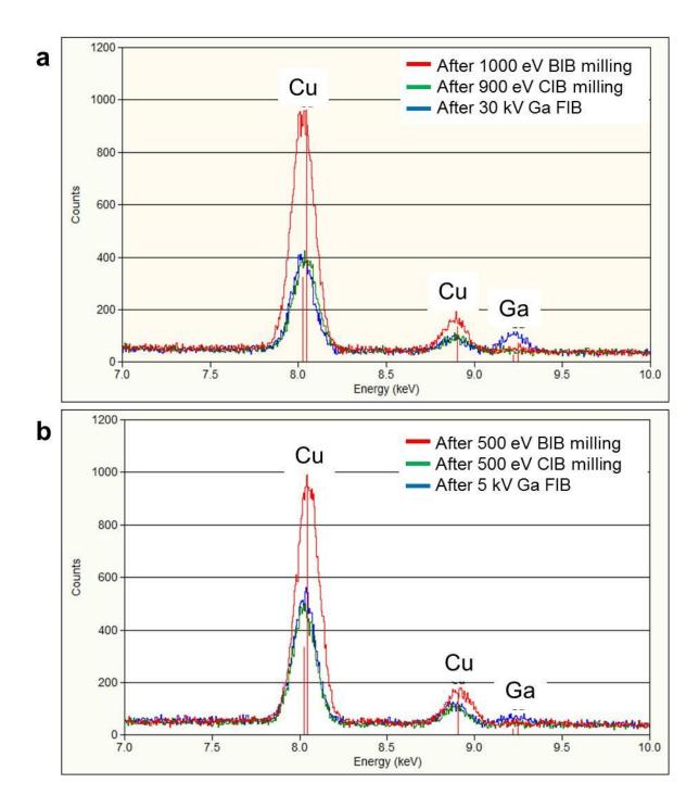
**Figure 2.** EDS using 300 kV accelerating voltage of Si specimens prepared by Ga FIB milling at 30 kV (a) and 5 kV (b) followed by BIB and CIB milling. Characteristic Cu K and Ga K peaks are shown.
