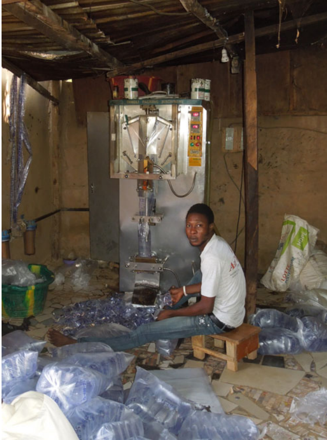
FIGURE 4 Automated sachet-filling machine in a private home.
