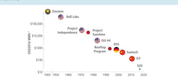
Box 16.4, Figure 1 | Milestones in the development of low-cost solar photovoltaics. Source: Nemet (2019).
