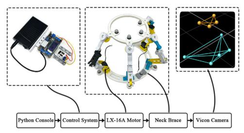
Figure 8. Control workflow for vicon validation.
