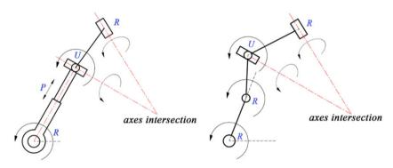
Figure 1. Component chain architectures with RPUR and RRUR.
