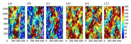
Figure 7. Wall-parallel views of small-box simulations. Colours are distance from the wall of the  $U^+ = 18$  isosurface. Flow is from the bottom upwards, and lengths are in wall units. (*a–c*) F950. Time between consecutive frames,  $u_\tau \Delta t/h \approx 0.52$ . (*d–f*) D950-0. Time between consecutive frames,  $u_\tau \Delta t/h \approx 0.30$ .
