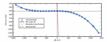
**Figure 2.** Change of focus vs. energy change (dE): In a Cc-corrected TEM electrons with a difference in energy of many hundreds of eV are focused to an identical image plane (blue curve) [5]. In a Cc-uncorrected TEM the defocus changes dramatically with change of energy (red dashed curve), consequently the resulting image contrast is strongly reduced.
