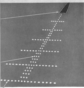
Three examples of G.E.C. Airport Lighting equipment designed for use in bad visibility are illustrated; the diagram showing how they are incorporated in a "Line and Bar approach" landing system.
