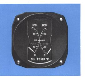
Model S. 127. Dual Ratiometer Indicator, comprising two 100° ratiometer movements housed in large-size S.A.E. case. For use in conjunction with thermometer bulbs, electrical oil pressure transmitters, electrical position indicators or any combination of two of these to indicate a variety of temperatures, pressures or positions
