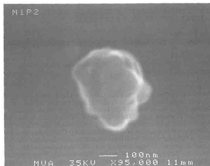
Figure 1. Secondary electron image of a GEM (mounted on a gold substrate).
