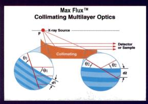
Graded d-spacing Max-Flux<sup>™</sup> Optic will collect a large solid angle of x-rays, filter and collimate to improve flux and resolution.
