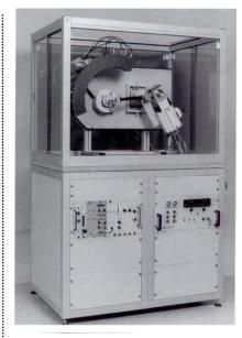
MPD Multi-Purpose X-ray Diffractometer
