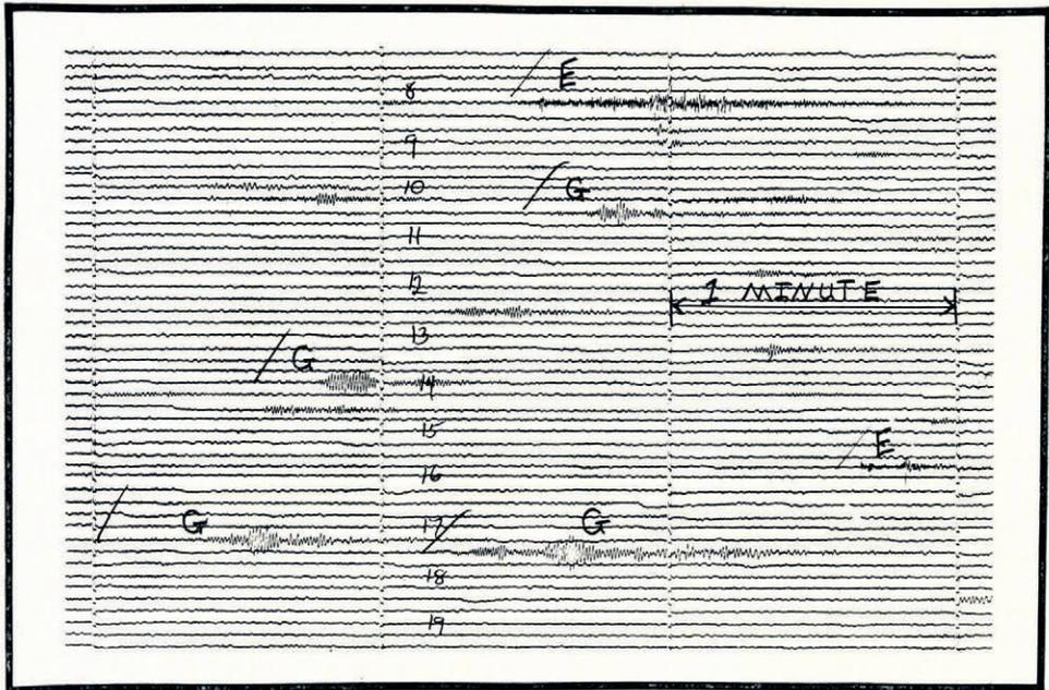
Fig. 4. Record sample from 28 May 1972. Signals marked "E" are earthquakes, the larger glacier signals are marked "G".
