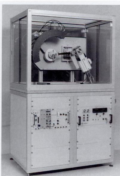
MPD Multi-Purpose X-ray Diffractometer
