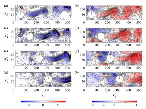
Figure 17. For  $S_3$ , a sequence ( $\Delta t^+ = 5.5$ ) of equatorial wall-parallel planes depicting the correlations of the instantaneous water fluctuating velocities ( $u_1u_2$ )<sup>+</sup> (a,c,e,g), and the streamwise water fluctuating velocities  $u_1^+$  (b,d,f,h). The hydrogel sphere is superposed as a filled white circle. Its initial orientation is indicated by a dashed line, while its changing orientation is indicated by a solid line. Note that the view is from the wall upwards.
