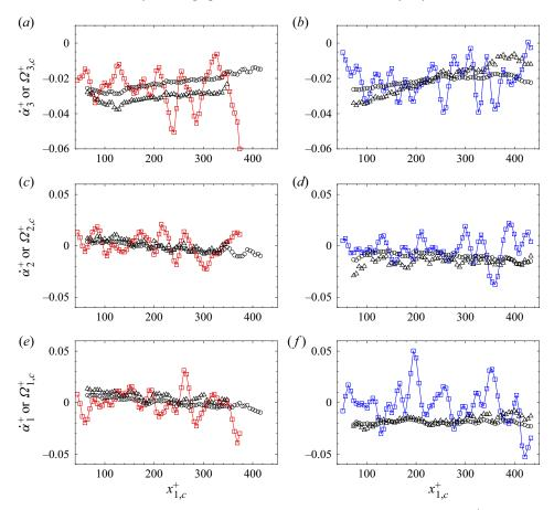
Figure 12. Instantaneous normalized angular velocities of the sphere and the water versus  $x_{1,c}^+$  for  $S_1$  (a,c,e) and  $S_2$  (b,d,f). Squares indicate sphere angular velocities  $\dot{\alpha}_i^+$  based on smoothed data. Water angular velocities at the sphere position are given for:  $\Omega_{i,c}^{v+}$ , circles; and  $\Omega_{i,c}^{c+}$ , triangles. Rotation is about: (a,b)  $x_3$ , (c,d)  $x_2$ , (e,f)  $x_1$ .
