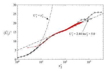
Figure 4. Semi-logarithmic plot of  $\langle \bar{U}_1 \rangle^+$  as a function of  $x_2^+$ . Present data: red squares denote  $Re_\theta = 850$ ; the dash-dot curve denotes the velocity profile in the viscous sublayer; the dashed line denotes the 'log-law'. Literature results (De Graaff & Eaton 2000): diamonds denote  $Re_\theta = 1430$ ; triangles denote  $Re_\theta = 5200$ .
