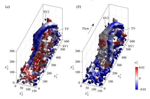
Figure 6. Example snapshot of Q-criterion iso-surfaces visualizing the coherent structures detected in the undisturbed TBL. Iso-surfaces are overlaid by (a) the normalized transverse vorticity  $\omega_1^+$ , and (b) the normalized streamwise vorticity  $\omega_3^+$ . An animation (supplementary movie 1) depicting the snapshot at different angles is available at https://doi.org/10.1017/jfm.2022.477.
