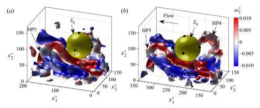
Figure 19. Close-up of vortical structures in the vicinity of  $S_4$ . Vortical structures were visualized by Q-criterion iso-surfaces that were overlaid by  $\omega_1^+$ . Snapshots in (a,b) correspond to figures 18(a,b).
