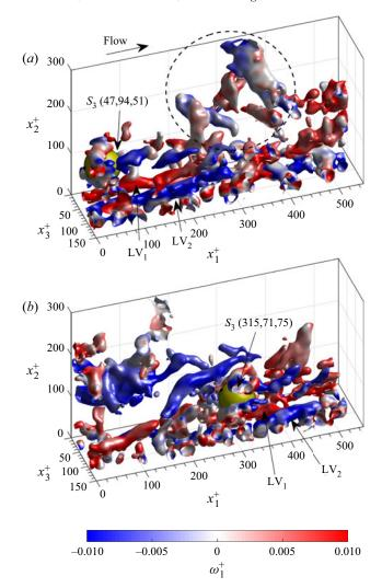
Figure 14. Two snapshots ( $\Delta t^+ = 16.7$ ) of the instantaneous vortical structures in the vicinity of  $S_3$  visualized by Q-criterion iso-surfaces overlaid by  $\omega_1^+$ . The sphere's surface is depicted in yellow, with black markers to indicate its change in orientation. Values in parentheses denote  $(x_{1,c}^+, x_{2,c}^+, x_{3,c}^+)$ . Supplementary movie 2 provides animations of the snapshot in (a) at different viewing angles.
