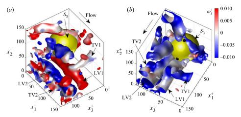
Figure 15. Close-up of the snapshot of sphere  $S_3$  in figure 14(a) at two different viewing angles. Vortical structures are visualized by Q-criterion iso-surfaces overlaid by (a)  $\omega_1^+$ , and (b)  $\omega_3^+$ . The sphere surface is depicted in yellow, with black markers indicating its orientation.
