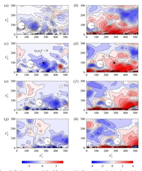
Figure 16. For  $S_3$ , a sequence  $(\Delta t^+ = 5.5)$  of equatorial wall-normal planes depicting the correlations of instantaneous water fluctuating velocities  $(u_1u_2)^+$  (a,c,e,g), and the streamwise water velocity fluctuating velocities  $u_1^+(b,d,f,h)$ . The hydrogel sphere is depicted as a filled white circle. Its initial orientation is indicated by a dashed line, while its changing orientation is indicated by a solid line.
