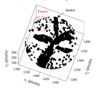
Figure 3. Example of the binarized reconstructed light intensity field confined within the determined sphere boundary. Spokes are numbered from 1 to 5. Tracer particles at the perimeter of the sphere are shown as small black dots (examples within dashed red ellipse).
