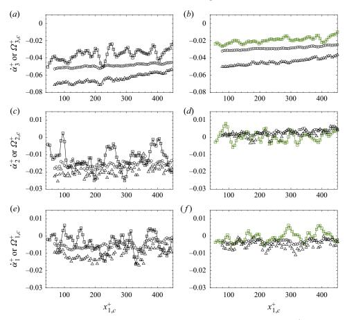
Figure 13. Instantaneous normalized angular velocities of the sphere and the water versus  $x_{1,c}^+$  for  $S_3$  (a,c,e) and  $S_4$  (b,d,f). Squares indicate sphere angular velocities  $\dot{\alpha}_i^+$ , based on smoothed data. Water angular velocities at the sphere position are given for:  $\Omega_{i,c}^{v+}$ , circles; and  $\Omega_{i,c}^{c+}$ , triangles. Rotation is about: (a,b)  $x_3$ , (c,d)  $x_2$ , (e,f)  $x_1$ .
