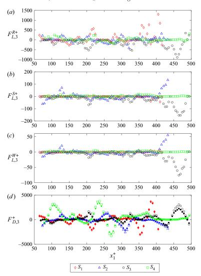
Figure 22. The instantaneous normalized transverse components of (a) the Magnus force, (b) the shear-induced lift force, (c) the wall-induced lift force, and (c) the drag force, acting on the spheres. Solid symbols in (d) denote values according to the standard drag relation. Note that the y-axis ranges are different.
