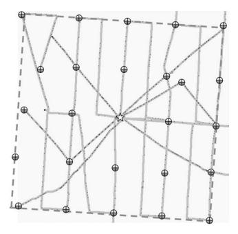
**Fig. 2.** The track lines of the roving GPS survey in the Dome A region. The rectangular region of interest, indicated using a dashed line, is the predefined area  $(20 \times 20 \, \text{km})$  of the survey. The base camp of the expedition team is at the center of the area. The circles with crosses denote the location of static GPS checkpoint measurements, taken over periods of at least  $20 \, \text{min}$ .
