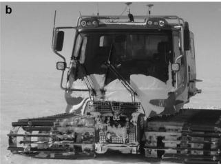
**Fig. 1.** (a) The reference GPS station at the base camp. The green cabin is the living quarters, the GPS antenna is installed on a tripod and the radio antenna is on the top of the cabin. (b) The dual roving GPS receivers mounted on the Pisten Bully 300 over-snow vehicle. The two antennas are on top of the vehicle and the radio antenna is on the top-left side of the cab.
