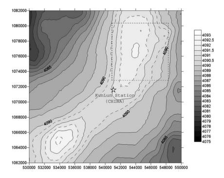
**Fig. 3.** Map of surface topography over the Dome A region surveyed by the 24th Chinese Antarctic National Research Expedition (CHINARE) in January 2008. Heights are with respect to the WGS84 system. The map is projected into the Universal Transverse Mercator (UTM) 43S zone. Contour interval is 1 m (with dashed contours at 0.5 m). The dashed rectangle covering the northern peak is the 64 km<sup>2</sup> area surveyed in early 2005 (Zhang and others, 2007).
