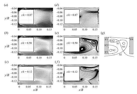
Figure 16. (a-c) Time-averaged velocity field  $(\bar{u}, \bar{v})$  and (d-f) corresponding streamlines in the xy-plane at vertical positions (a,d) z/k = 0.87, (b,e) z/k = 0.50 and (c,f) z/k = 0.12 for test case SUB2. Panel (g) is the interpreted flow topology of panel (e).
