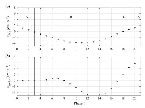
Figure 18. (a) Phase-averaged lateral velocity  $v_{PA,i}$  at y = 0, x/B = 0.1 and z/k = 0.5 as a function of phase i. (b) Lateral velocity averaged over the cavity length,  $v_{cavity}$ , as a function of the phase at z/k = 0.5. The letters A, B and C refer to the three different topologies that succeed during the passage of the structure.
