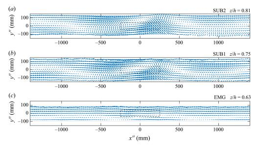
Figure 11. Velocity field ( $u_{EA} - U_c$ ,  $v_{EA}$ ) of the ensemble-averaged field obtained by PRT in the horizontal plane for test case (a) SUB2 at z/h = 0.81, (b) SUB1 at z/h = 0.75 and (c) EMG at z/h = 0.63. The dashed rectangle indicates the size of the template.
