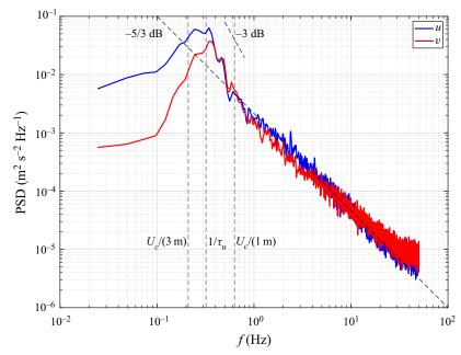
Figure 14. Power spectral density (PSD) of the fluctuations of the longitudinal (blue line) and lateral (red line) velocity for test case SUB2 at z/h = 0.81, y/B = 0.035 and x/B = 0.11. The vertical dotted lines depict the size range of the coherent structures between 1 and 3 m (converted to frequency using  $U_c$  as convection velocity), and the integral time scale  $\tau_u$  inferred from the auto-correlation of u(t) (figure 2).
