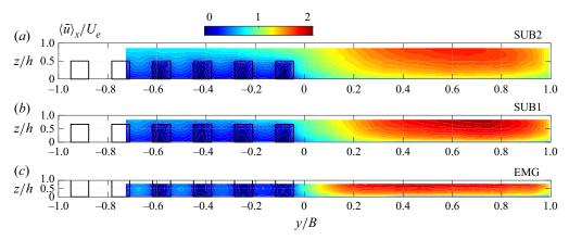
Figure 3. Cross-sectional distribution of double-averaged longitudinal velocity  $\langle \bar{u} \rangle_x$  for test cases SUB2, SUB1 and EMG.
