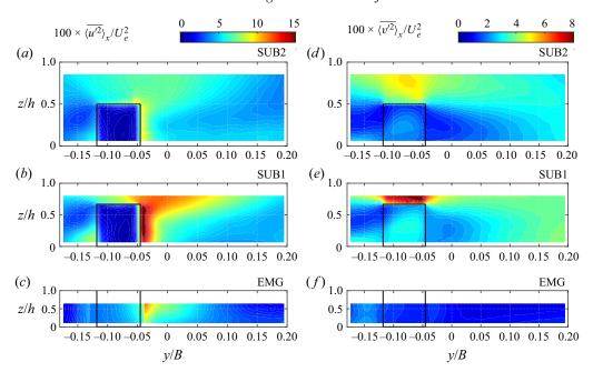
Figure 5. (*a–c*) Longitudinal and (*d–f*) lateral *x*-averaged turbulent normal stress in the *yz*-plane around the interface for test cases SUB2, SUB1 and EMG.
