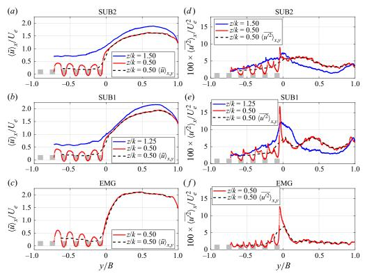
Figure 4. (a-c) Lateral profiles of time- and x-averaged longitudinal velocity (blue and red lines) and time-, x- and y-averaged longitudinal velocity (dashed black line) for the three test cases. (d-f) Same as panels (a-c) but for the longitudinal turbulent normal stress.
