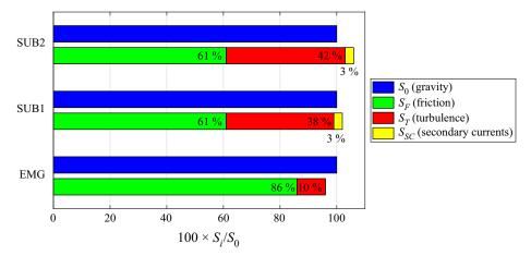
Figure 8. Momentum balance in the smooth subsection of the channel for the three test cases. The bars represent the different terms of (4.1), all normalised by the slope  $S_0$  and multiplied by 100. The blue bar is the slope itself (left-hand side of (4.1)), the green bar is the friction on the bottom and side wall, the red bar is the lateral exchange at y = 0 due to turbulence and the yellow bar the lateral exchange at y = 0 due to secondary currents.
