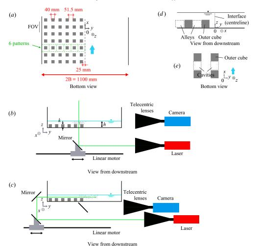
Figure 1. (a) Bottom view of the channel; the vertical line on the left side indicates the streamwise extent of the field of view (FOV) of the camera. (b) Experimental set-up for lateral and (c) for vertical scanning 3-D-2-C PIV. (d,e) Definition of some flow regions and references used in the text.
