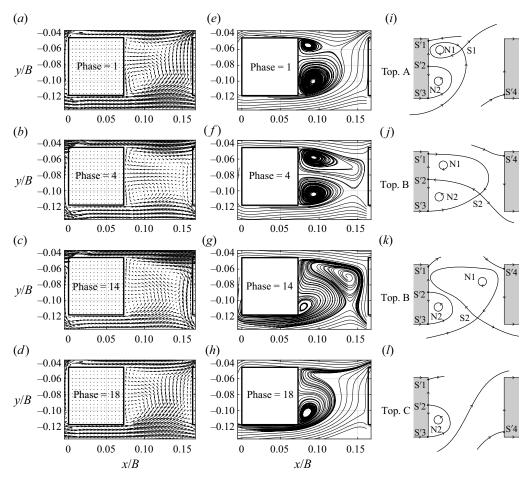
Figure 19. Phase-averaged flow field in the *xy*-plane obtained for the phase i = 1, 4, 14 and 18 for test case SUB2 at z/k = 0.5: (a-d)  $(u_{PA,i}, v_{PA,i})$ -field, (e-h) streamlines, (i-l) flow topology.
