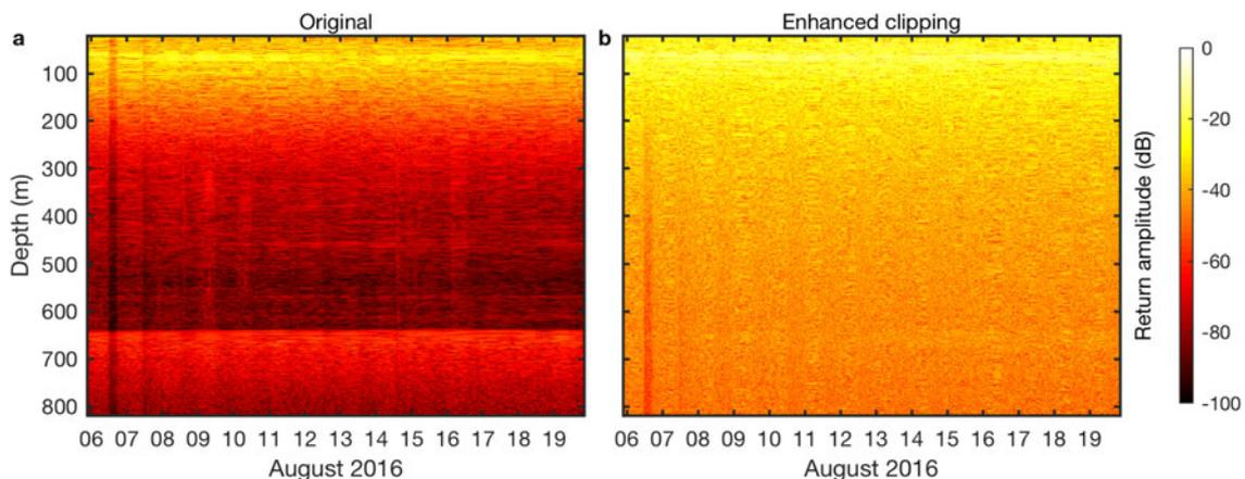
**Fig. 5.** Return amplitude at Helheim site H3Y16 (a) using the last quarter of the deramped chirp (350–400 MHz band) which avoids clipping, and (b) the full deramped chirp (200–400 MHz band) with clipping sufficiently enhanced to highlight how clipping obscures the bed return signal with artifacts.
