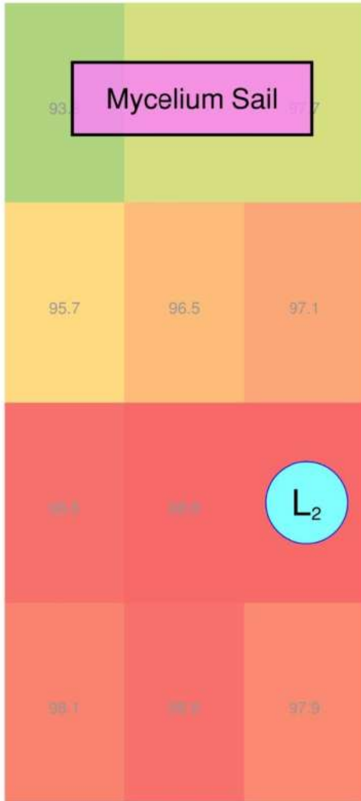
Figure 12: Measured dB(A), Source further away from sail (L2), Source: Albert Dwan (Arup)
