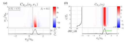
FIGURE 3. (a) Gyrotropic field–particle correlation signature  $C_{E_{\parallel}}(v_{\parallel}, v_{\perp})$  at  $t/T_0 = 6.75$  and (b) timestack plot  $C_{E_{\parallel}}(v_{\parallel}, t)$  of a driven, damped wave simulation with  $\beta_i = 0.1$ ,  $k_{\perp}\rho_i = 8$  and a correlation interval of  $\tau/T_0 = 1$ . In the time-integrated subpanel (below) in (b), the full-width at half-maximum (FWHM) of the positive portion of the bipolar signature is indicated.
