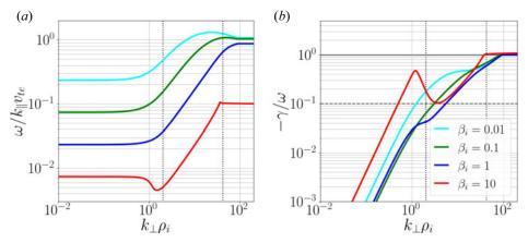
FIGURE 2. Linear Vlasov–Maxwell dispersion relation for plasmas with  $T_i/T_e = 1$ ,  $m_i/m_e = 1836$ , and  $\beta_i = 0.01$  (cyan), 0.1 (green), 1 (blue) and 10 (red). (a) Parallel phase velocity normalized to the electron thermal velocity  $\omega/k_{\parallel}v_{te}$ . (b) Normalized damping rate  $-\gamma/\omega$ , with the onset of strong damping  $(-\gamma/\omega \gtrsim 0.1)$  marked by a horizontal dashed line.
