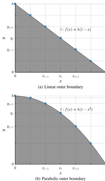
FIGURE 2. Geometries with (a) linear outer boundary and (b) parabolic outer boundary and their corresponding grids.
