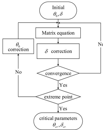
FIGURE 1. Flow chart for the indirect numerical method.
