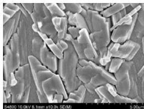
Figure 4. SEM image of MOCVD-grown SnS deposited at 470°C on to Mo.
